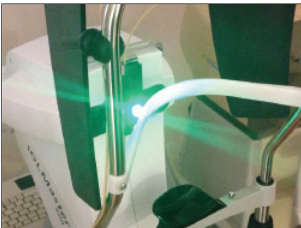
Figure 1. The IOLMaster 500 with ORI: The green light is used to ensure alignment for reference imaging.
